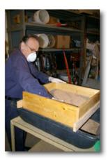
sorted by size into two separate plastic tubs. The two sizes would form the basis of the coarse and fine grade soil mixtures that were being made.
